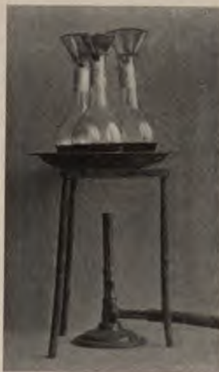
Fig. 97.—"Pancreatic" reaction flasks fitted with funnel condensers on a sand-bath.
